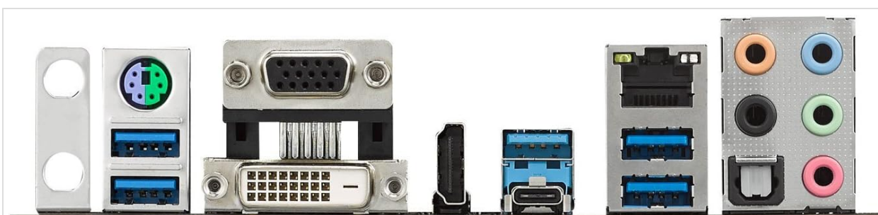
Figure 3: Detailed view of the rear I/O panel, featuring USB ports, display outputs (HDMI, DVI-D, D-Sub), Ethernet, and audio jacks.
