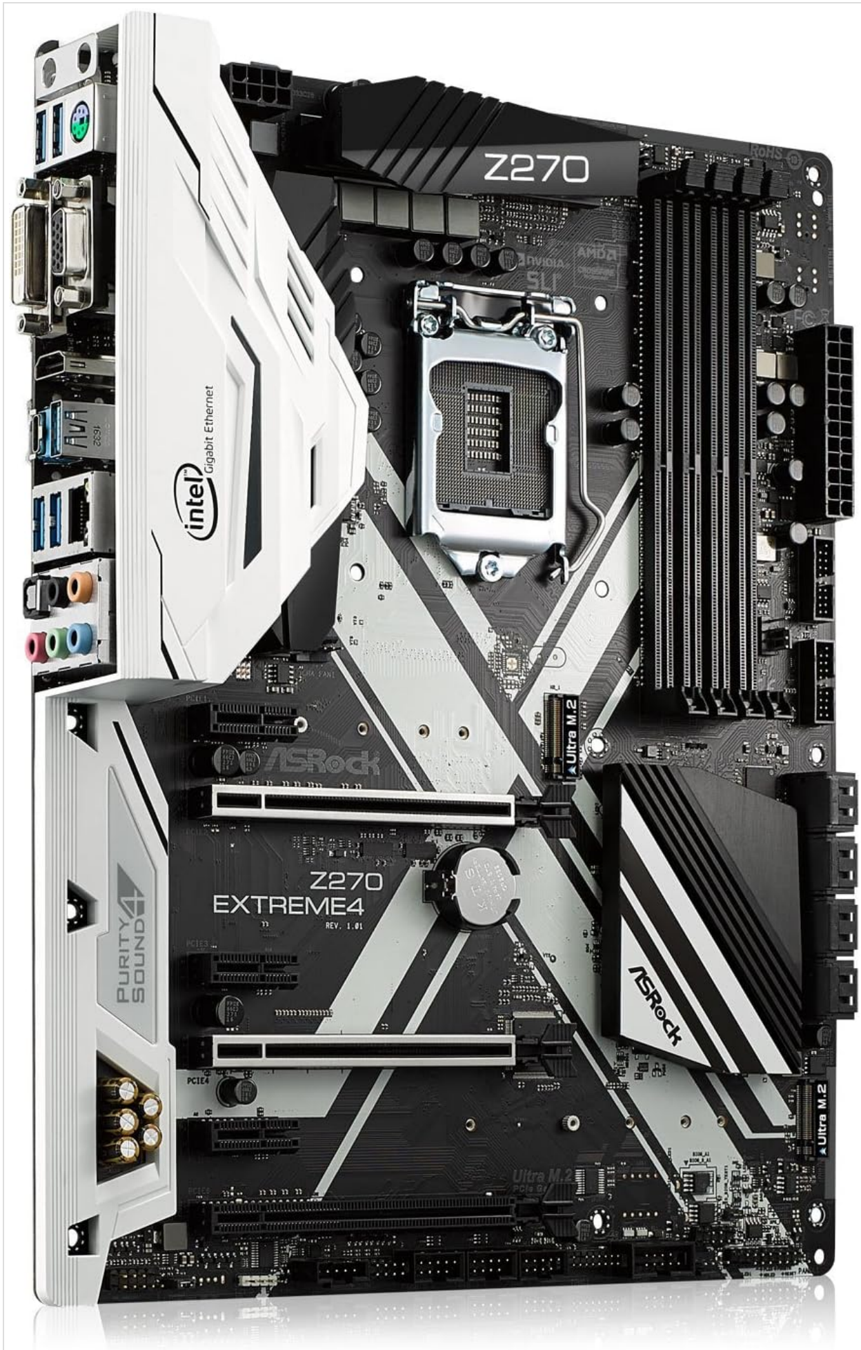
Figure 1: Top-down view of the ASRock Z270 EXTREME4 motherboard, showing the CPU socket, RAM slots, PCIe slots, and various headers.
