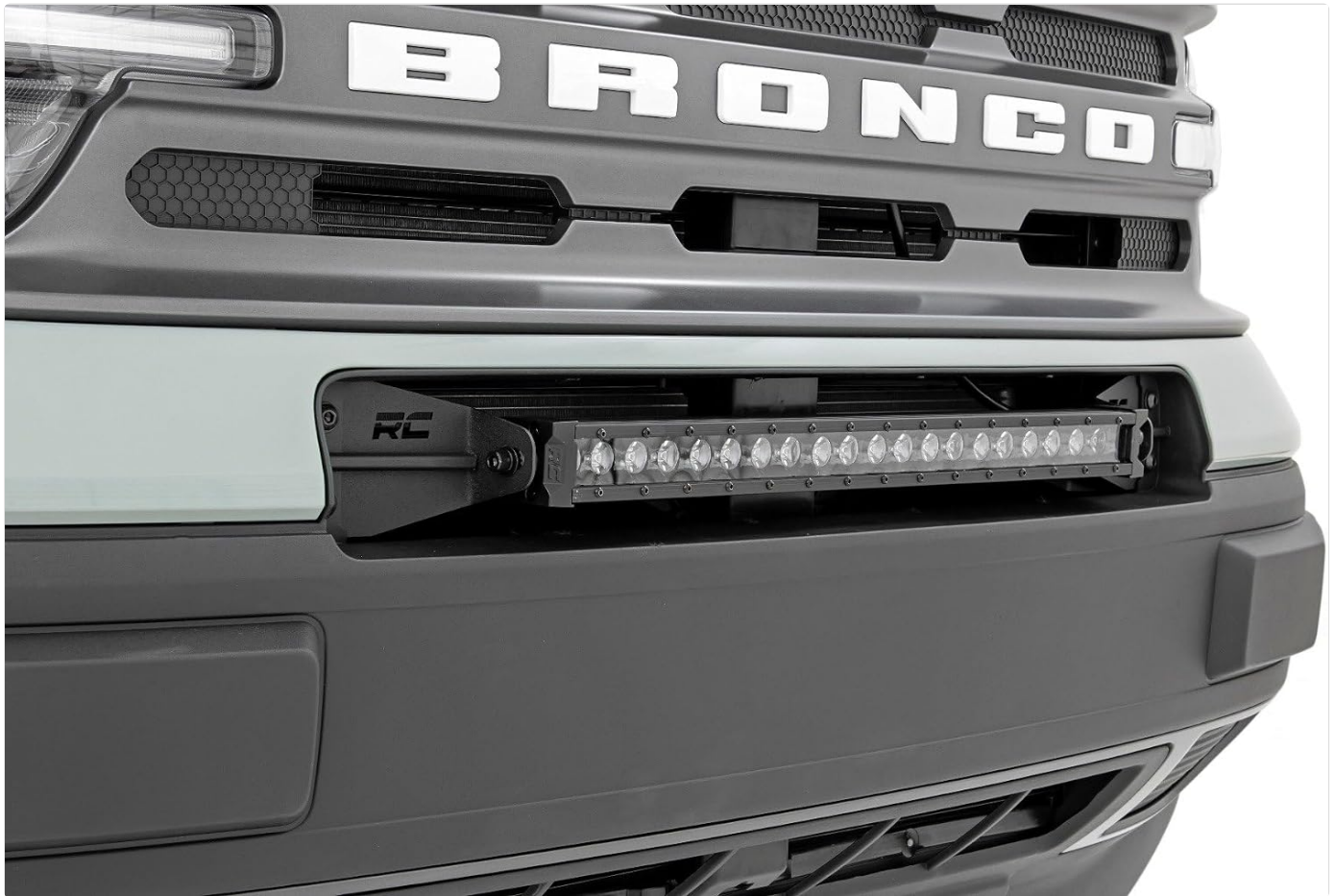
Image 3: Light Bar Installed on Vehicle (Daytime)
