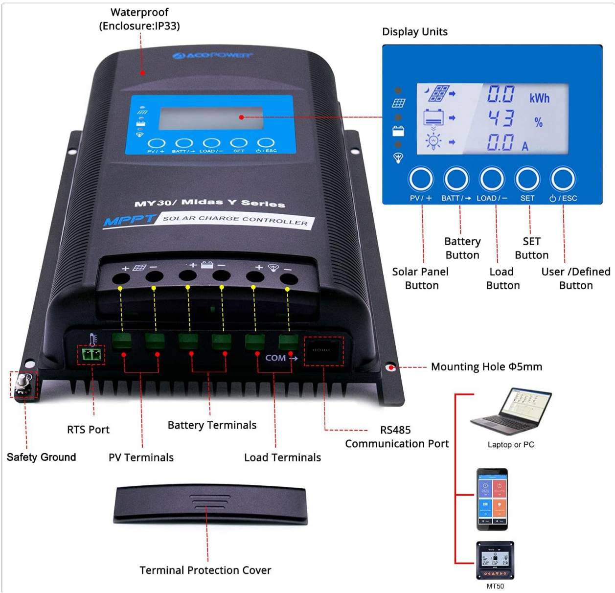
Figure 3.2: Component diagram of the controller, highlighting ports and buttons.
