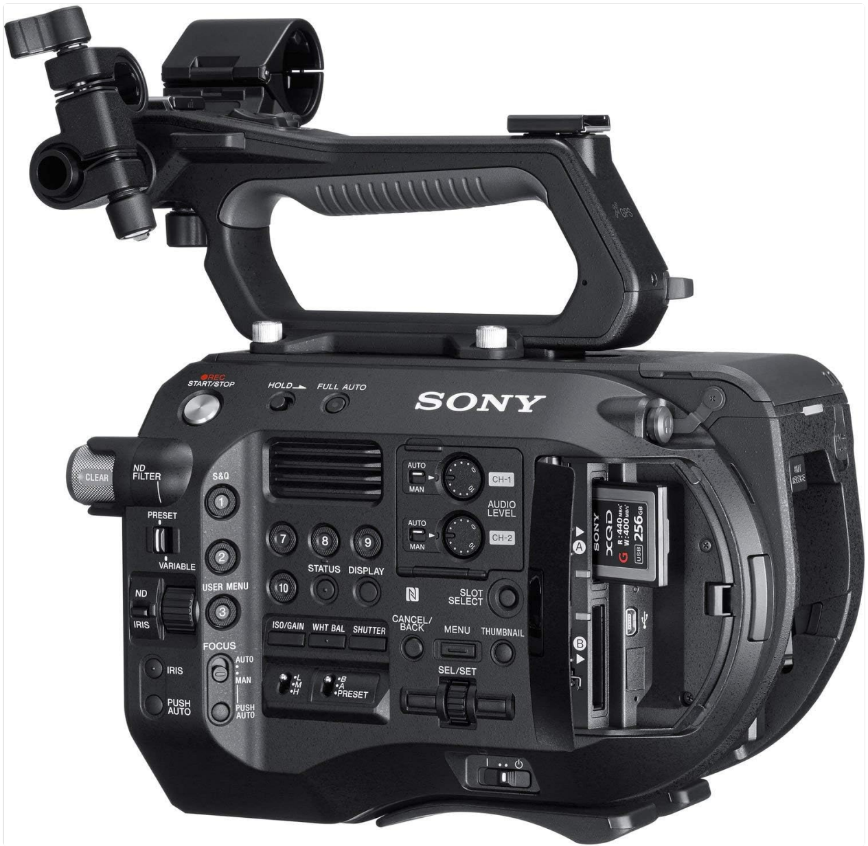
Figure 2.3: Side view showing the open XQD card slot.
