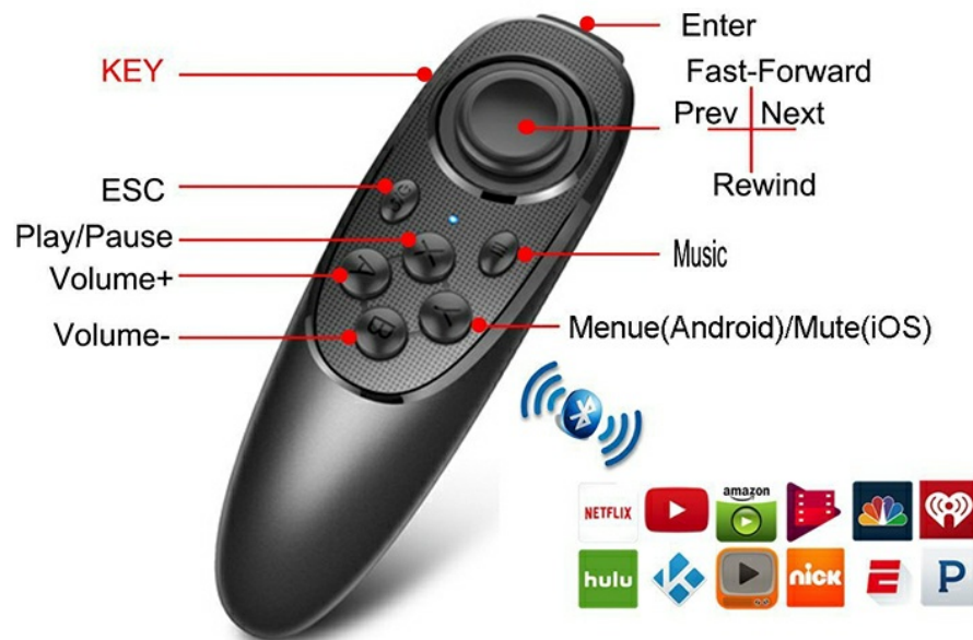
Image 5.4: Diagram detailing mouse functions in KEY Mode, where the joystick controls cursor movement and buttons act as left/right clicks. This function is available for Android, Windows, SmartTV, and TV Box devices.
