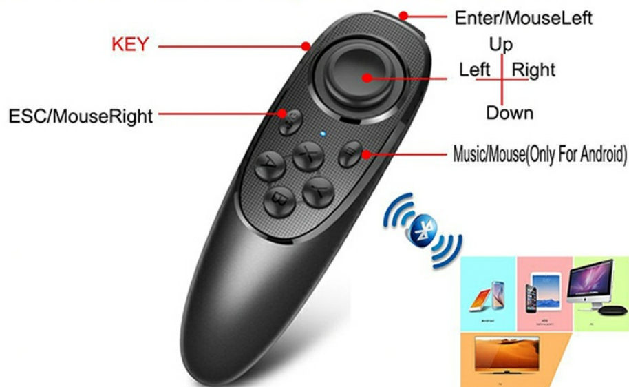
Image 5.5: Diagram illustrating how the controller facilitates page flipping for iReader (KEY Mode with A and B keys),
