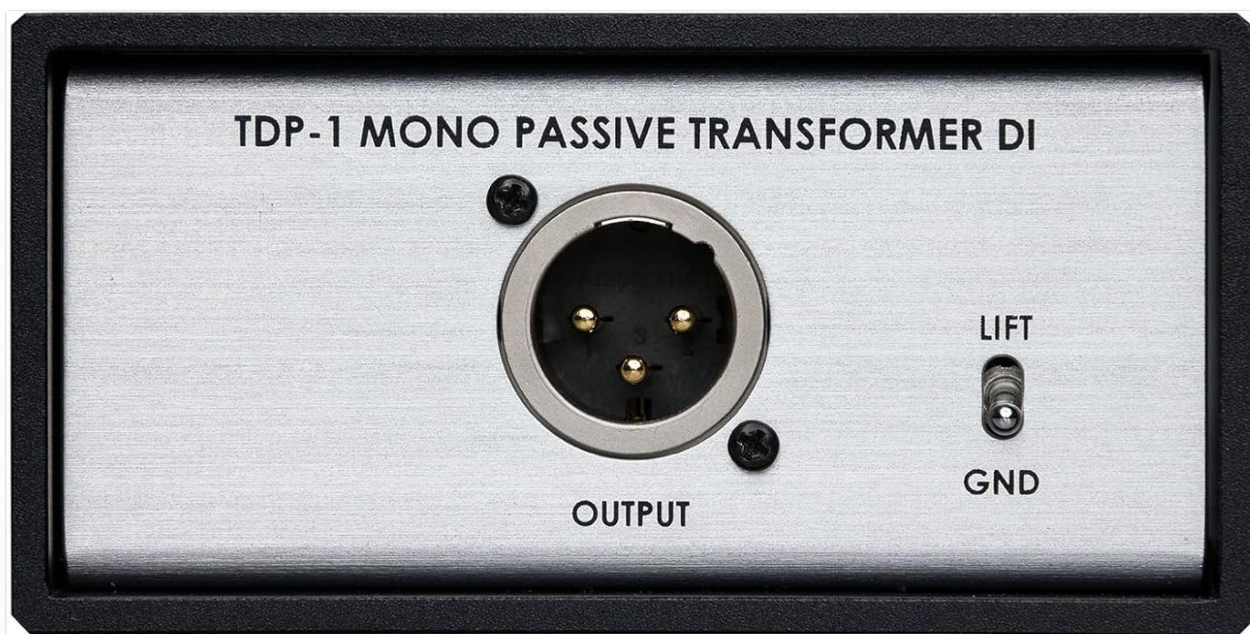
Figure 2: Output Panel. This close-up view highlights the XLR output connector and the Ground Lift switch. The XLR output is a standard 3-pin male connector for balanced audio signals. The Ground Lift switch helps to break ground loops, reducing hum and noise.
