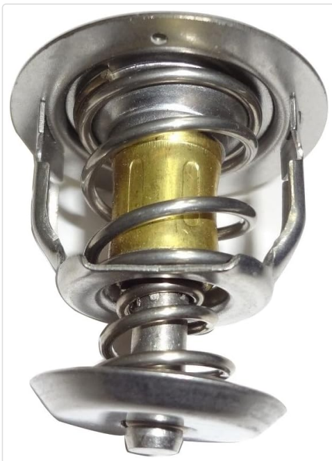
Image 2: A side view of the thermostat, showing its internal spring mechanism and wax pellet, which expands and contracts to open and close the valve.
