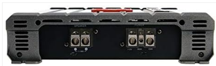
Figure 4.1: Rear panel of the CB1-2500D amplifier showing power, speaker, and input connections.
