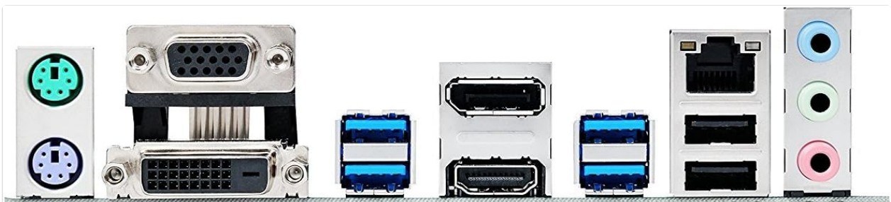
Figure 4.3: Close-up of the rear I/O panel, displaying the PS/2 ports, VGA, DVI, HDMI, USB 3.0, LAN, and audio jacks.
