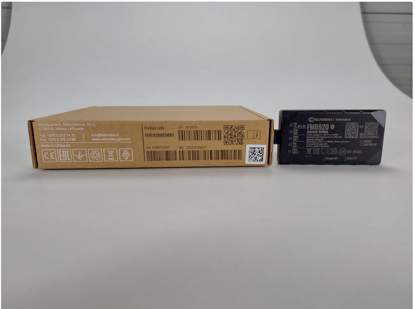
Figure 1: Teltonika FMB920 device alongside its retail packaging, showing the compact size of the tracker and the information printed on the box.
