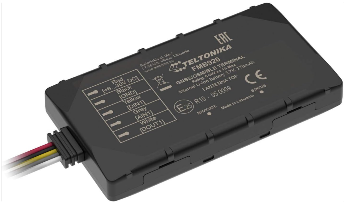
Figure 2: Top view of the Teltonika FMB920 showing the wiring harness with color-coded wires and their respective functions (Red for Power, Black for Ground, Yellow for Digital Input, Grey for Analog Input, White for Digital Output).
