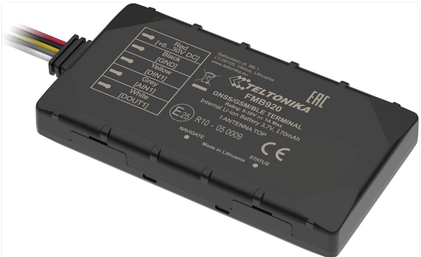
Figure 2: Top view of the Teltonika FMB920 showing the wiring harness with color-coded wires and their respective functions (Red for Power, Black for Ground, Yellow for Digital Input, Grey for Analog Input, White for Digital Output).
