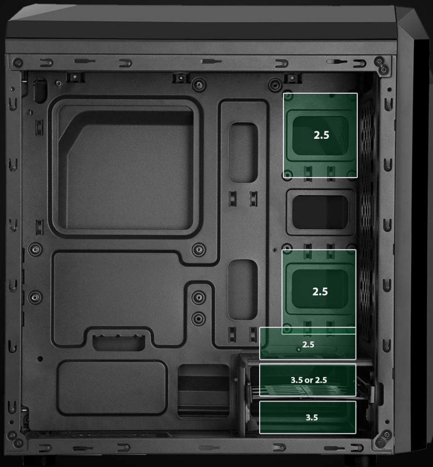
Figure 3.2: Internal view showing the flexible storage options for 2.5-inch and 3.5-inch drives within the case.
