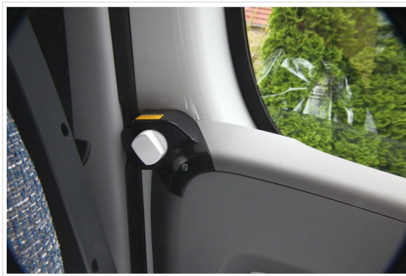
Image: HEOSafe lock installed on the vehicle's door frame, showing its position near the window.
