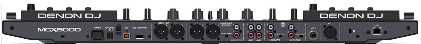
Figure 3: Rear view of the Denon MCX8000, detailing the various input and output ports including XLR, RCA, USB, and power connections.
