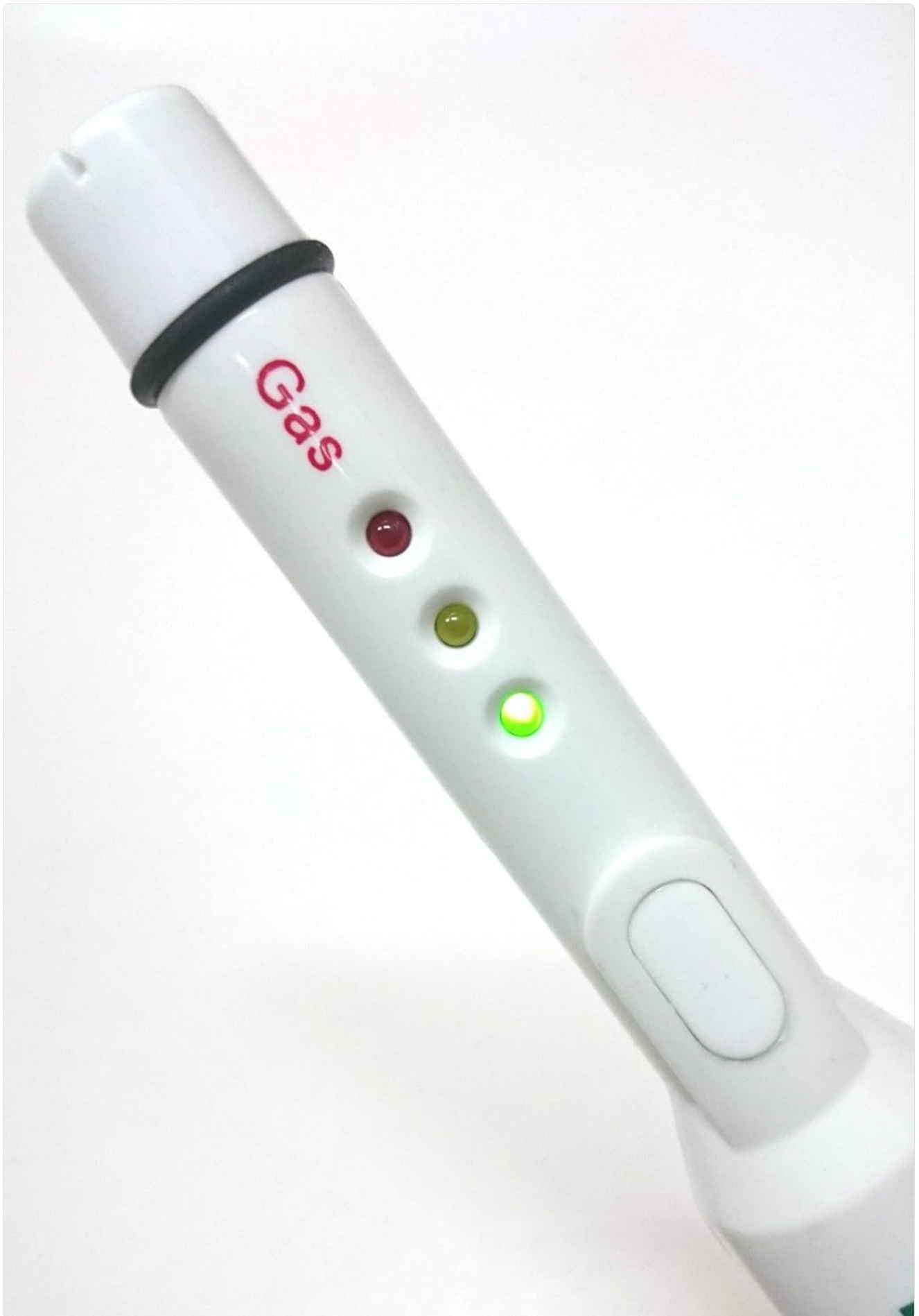
Figure 4.3: Side view of the GA0080, illustrating the three LED indicators (green, yellow, red) for visual alarm signals.
