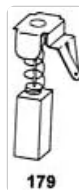
Image 3.1: A simplified diagram illustrating the components of a carbon brush assembly, including the brush, spring, and connector. This helps visualize the parts involved in installation.
