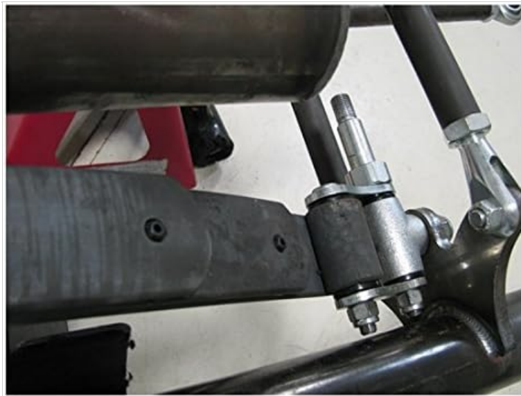
Image: A detailed view of the bracket's shock mounting points, showing how it integrates with the vehicle's suspension components on the frame rail.
