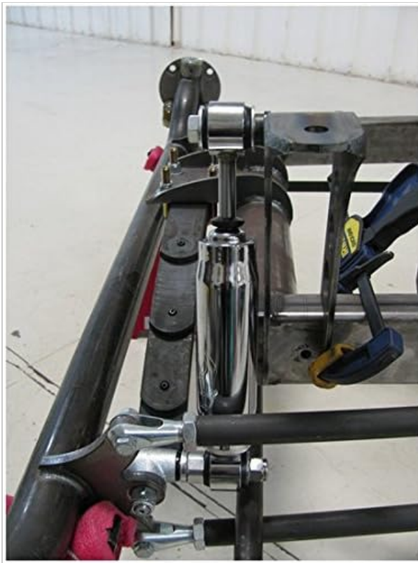
Image: The bracket with a shock absorber securely installed, illustrating the use of one of the dual shock mounting holes.
