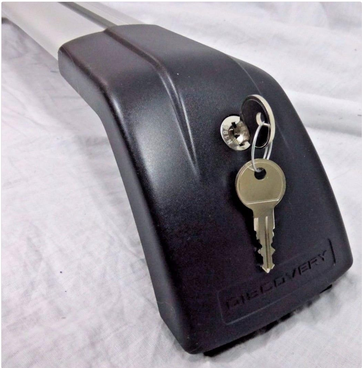
Figure 2: Detail of the locking mechanism on the crossbar end, showing the key inserted for securing the bar.
