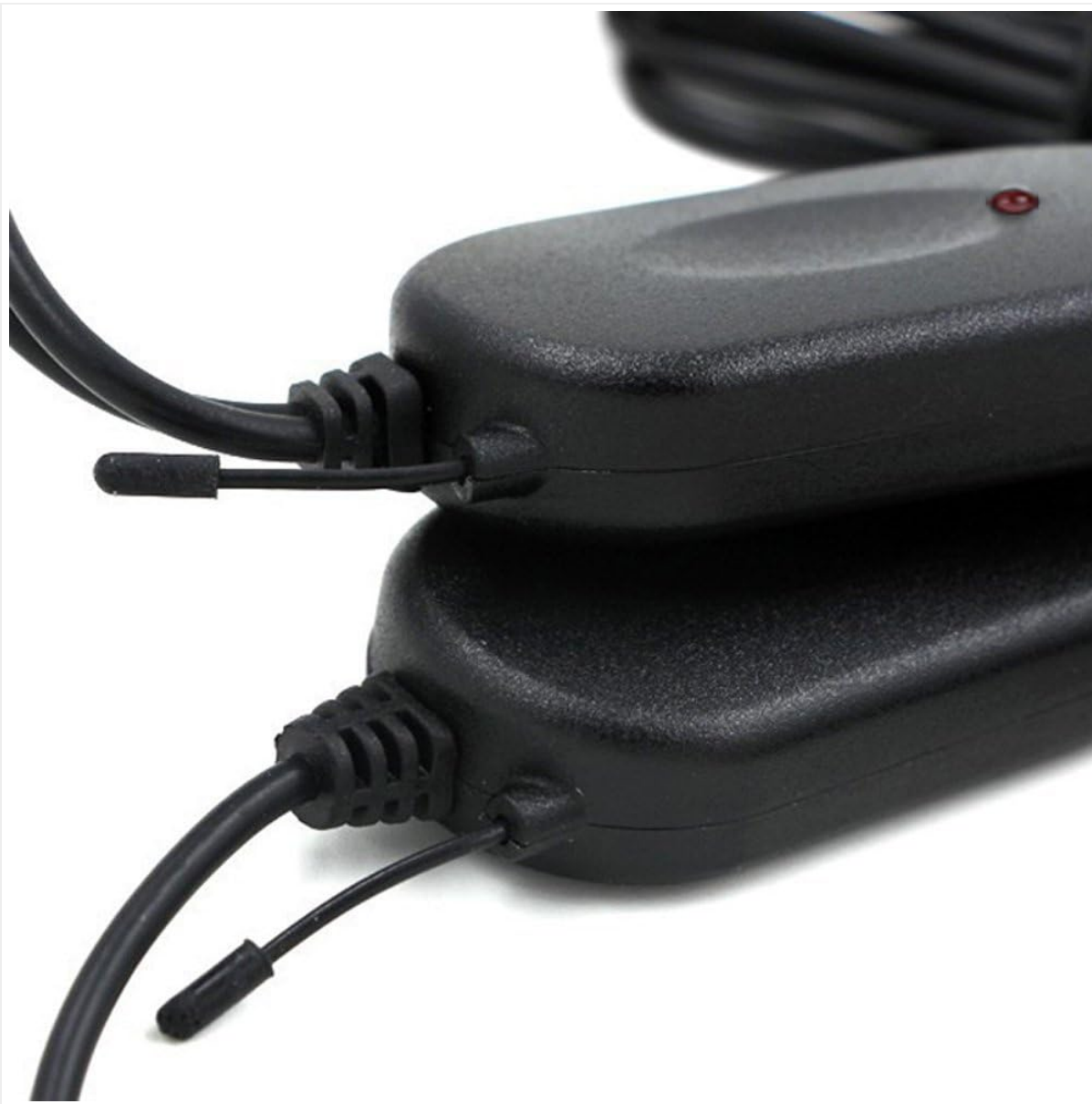
Figure 3.2: The 2.4G wireless transmitter and receiver units, responsible for wireless video signal transmission.
