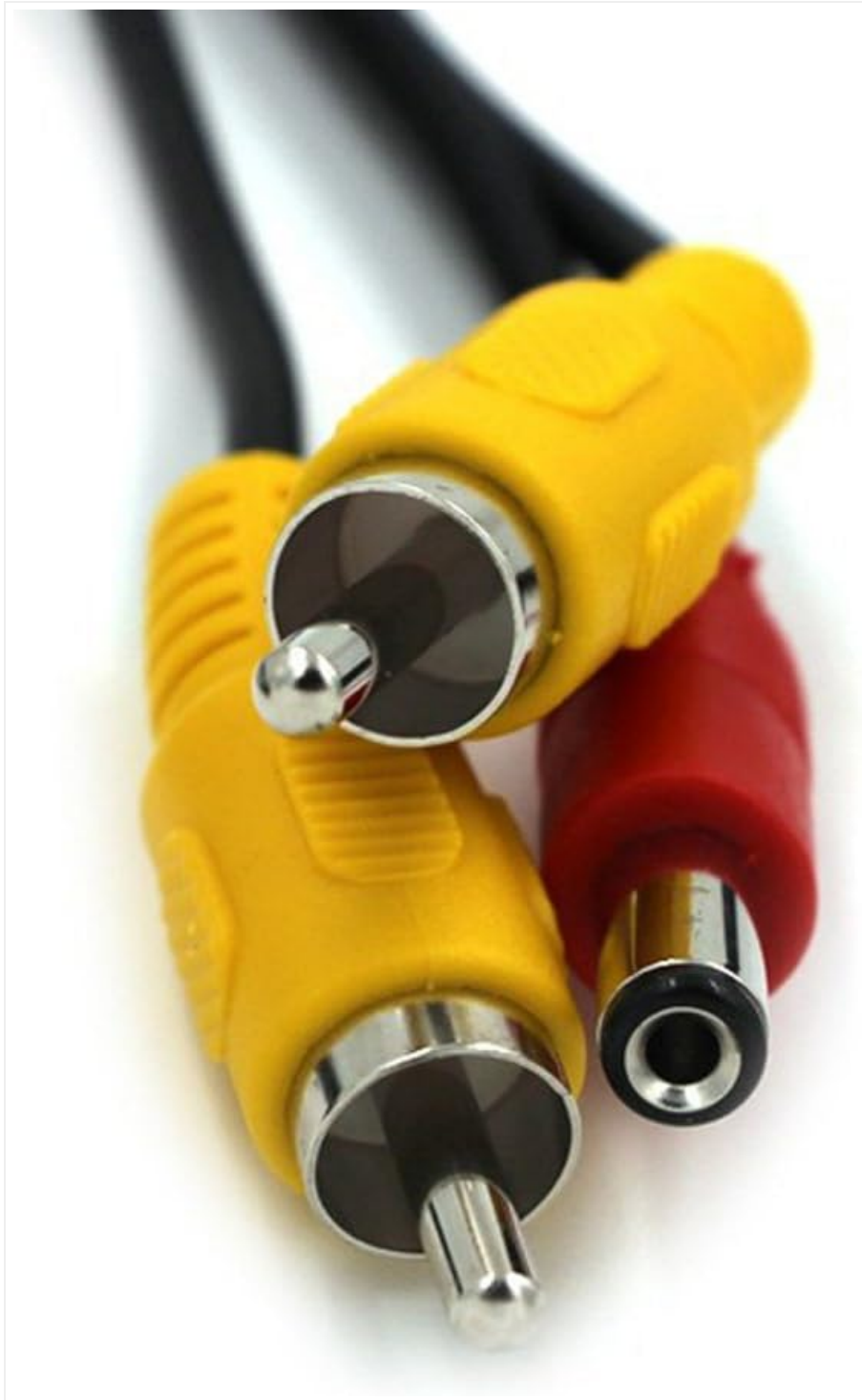
Figure 5.2: Detailed view of the RCA and power connections on the wireless transmitter and receiver units.
