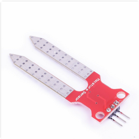
Image: Top view of the Cylewet Soil Moisture Sensor Module, showing the red PCB and the two conductive probes.
