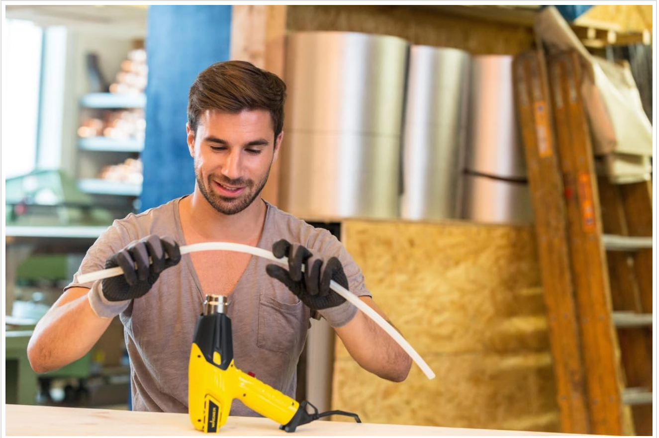
Figure 3: Demonstrating the heat gun's use for bending PVC pipes.
