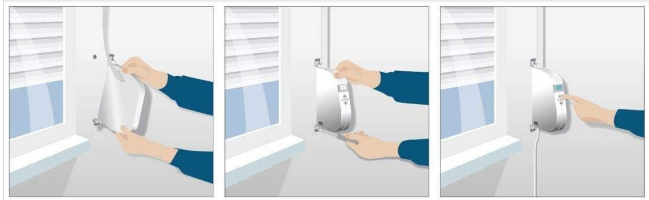
Figure 5.1: Step-by-step illustration of the eWickler eW920 installation process, from preparing the mounting area to securing the device and connecting the belt.
