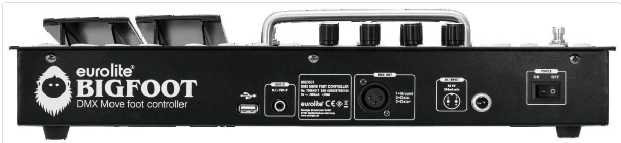
Figure 3.5: Rear panel of the controller, showing power input, DMX output, and USB port.
