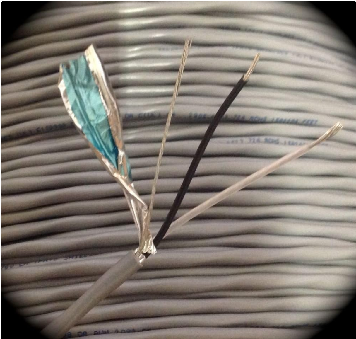
Figure 1: A section of the Belden 8760 cable with its outer PVC jacket removed, revealing the internal structure. Visible components include the twisted pair of insulated conductors, the metallic foil shield, and the bare drain wire. This image illustrates the cable's construction for proper termination.
