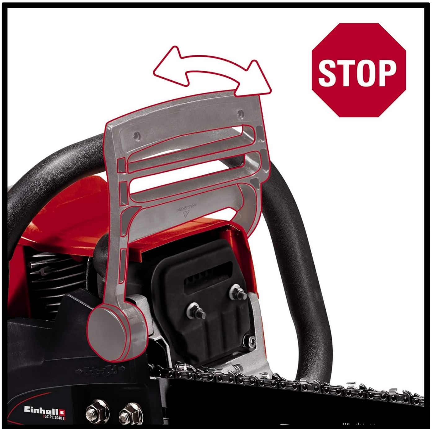
Figure 6: Visual representation of how to activate the immediate chain brake for emergency stops or when moving between cuts.
