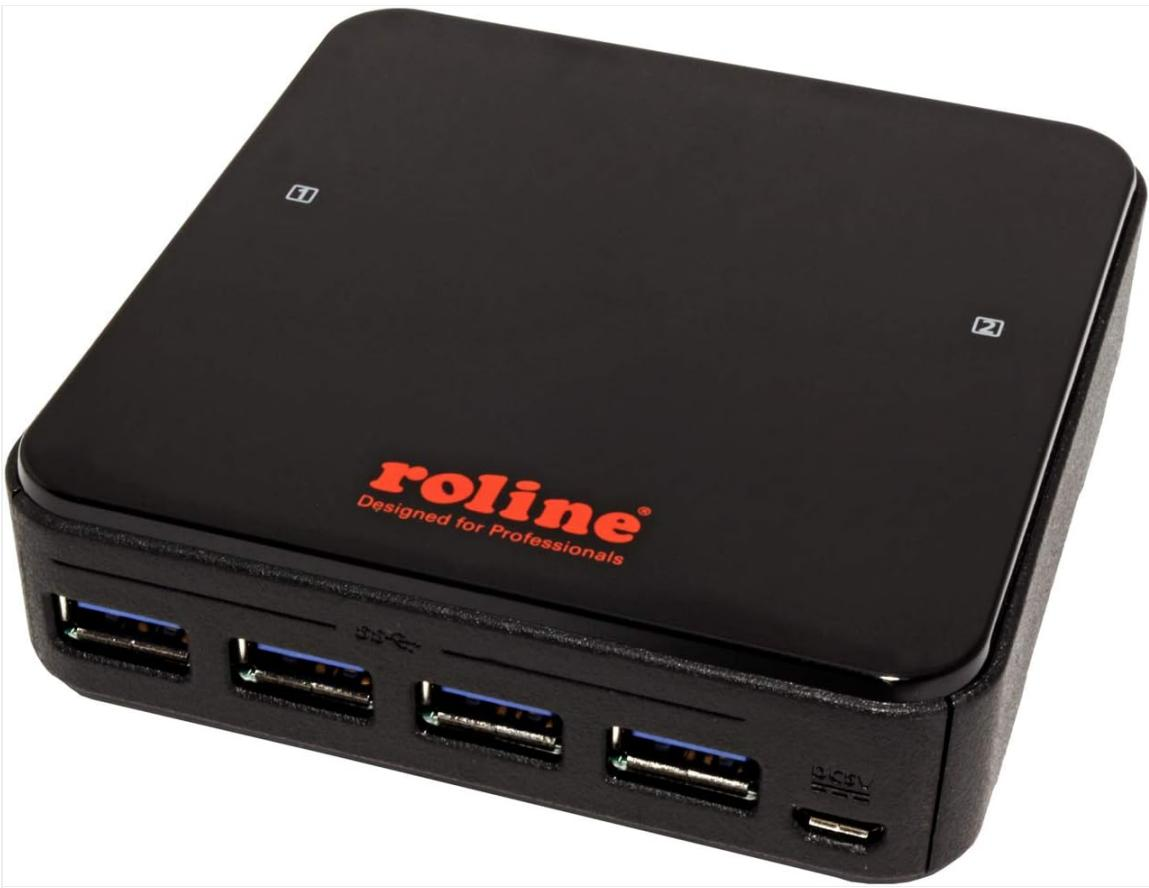
The front panel of the switch box, showing four blue USB 3.0 Type A output ports for connecting peripheral devices, and a micro-USB port for optional external power.
