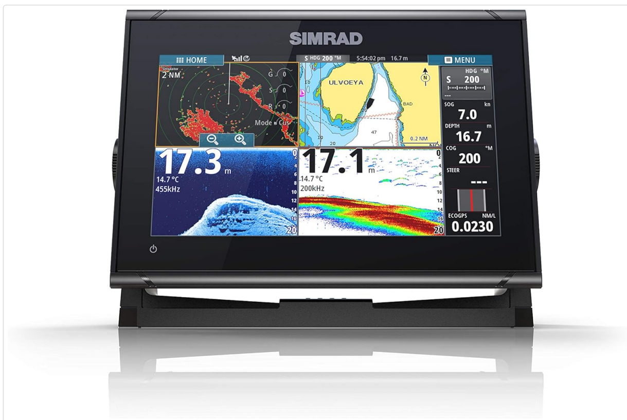
Figure 6: The Simrad GO9 XSE home screen, where the 'Radar' icon can be selected to access radar functions.
