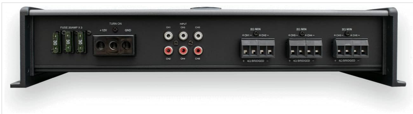
Image: Rear view of the Wet Sounds SYN-DX6 amplifier, detailing the power input (12V, GND, REM), RCA inputs (CH1-CH6), and speaker output terminals (2Ω MIN, 4Ω BRIDGED). This image is essential for correct wiring.
