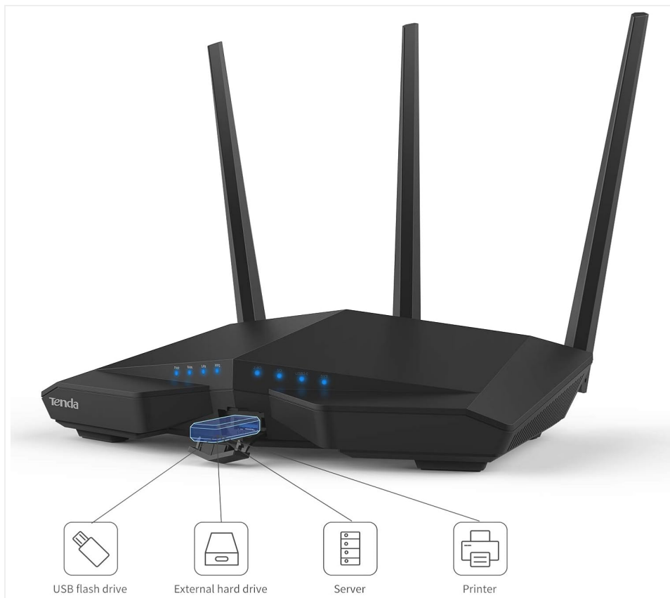
Figure 5.1: Illustration of the Tenda AC18 Router's USB 3.0 port, showing connectivity options for USB flash drives, external hard drives, servers, and printers.
