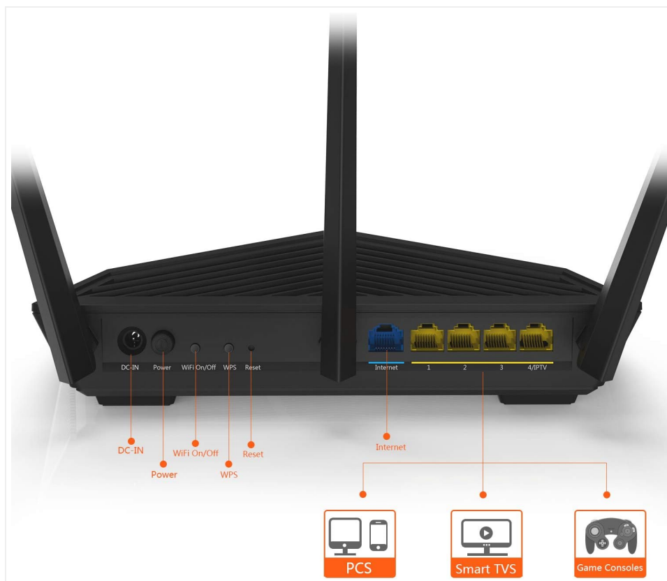
Figure 3.1: Rear view of the Tenda AC18 Router, highlighting the DC-IN, Power, WiFi On/Off, WPS, Reset buttons, and the Internet (WAN) and LAN ports.
