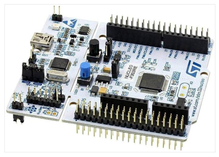
An overhead view of the STM32 Nucleo-64 Development Board, showcasing its various components including the STM32F303RE MCU, USB connector, ST-LINK debugger, and various pin headers for expansion.
