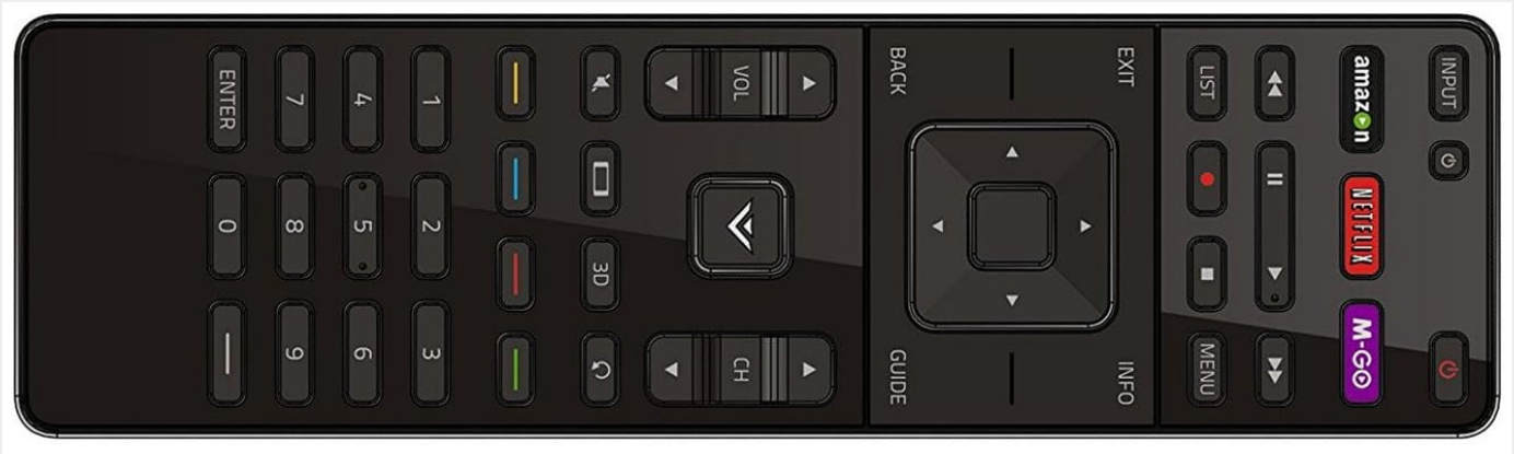
Figure 2: Top-down view of the Smartby XRT510 Remote Control, illustrating the layout of all buttons.
