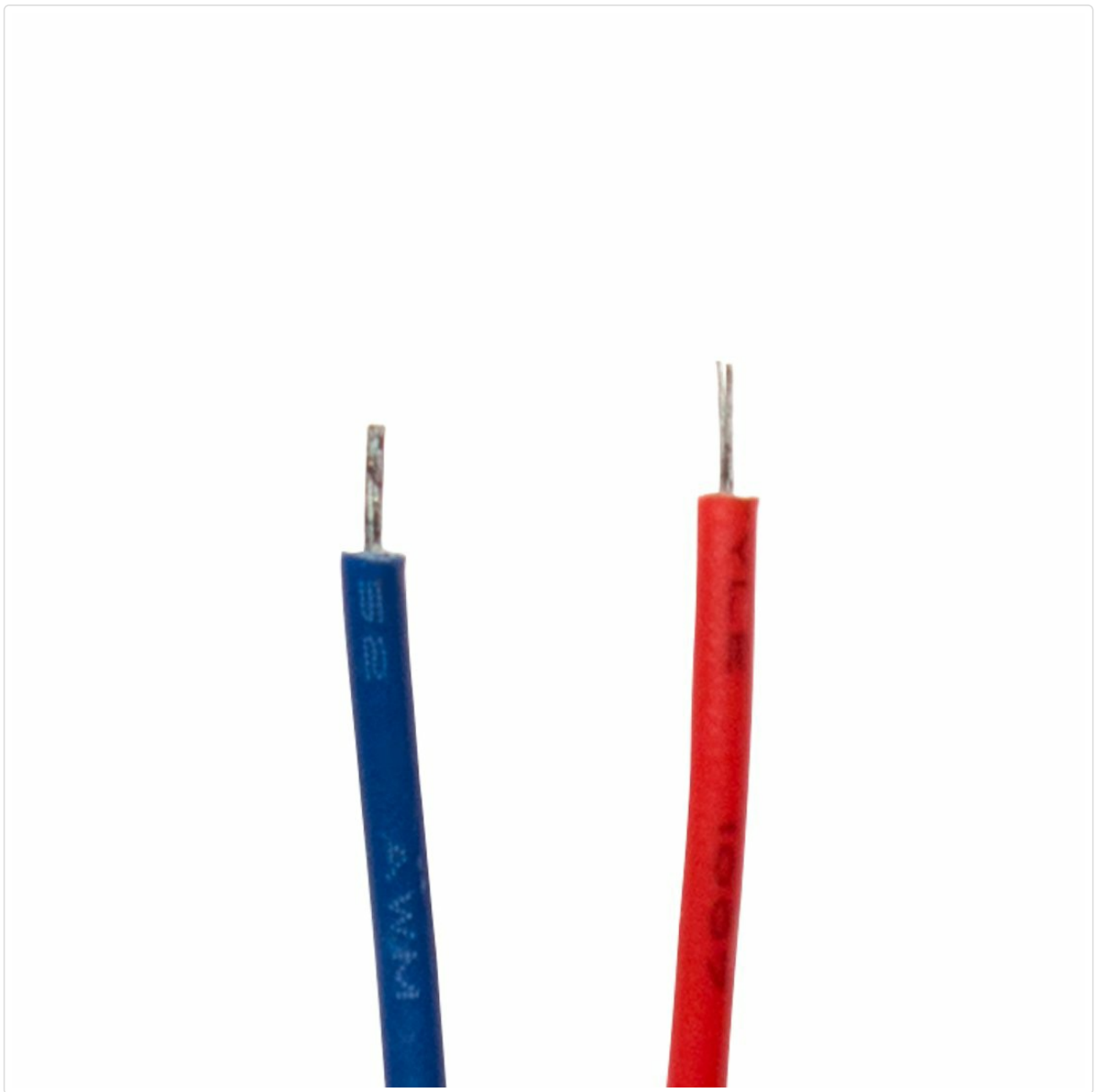
Figure 5: Close-up of the stripped ends of the red and blue power wires, ready for connection to a 5V DC power supply.
