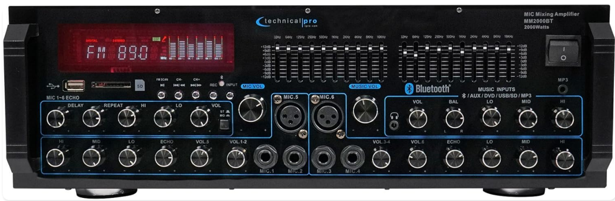
Figure 2: Detailed front panel layout of the MM2000BT, highlighting microphone and music input sections, equalizers, and master controls.
