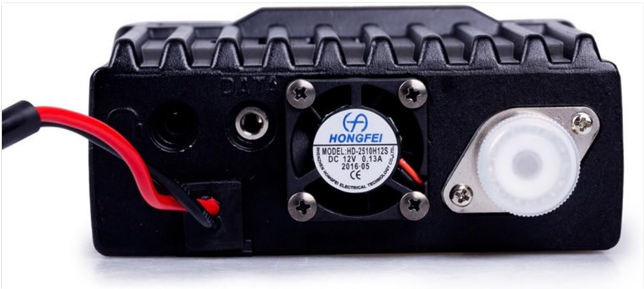
Figure 3.2: Rear view of the KT-7900D, showing the cooling fan and antenna port.
