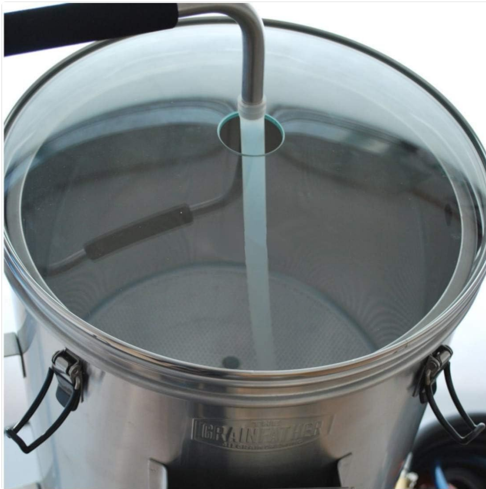
Figure 4: Interior view of the Grainfather, showing the grain basket in place and the recirculation arm returning wort to the top of the grain bed.
