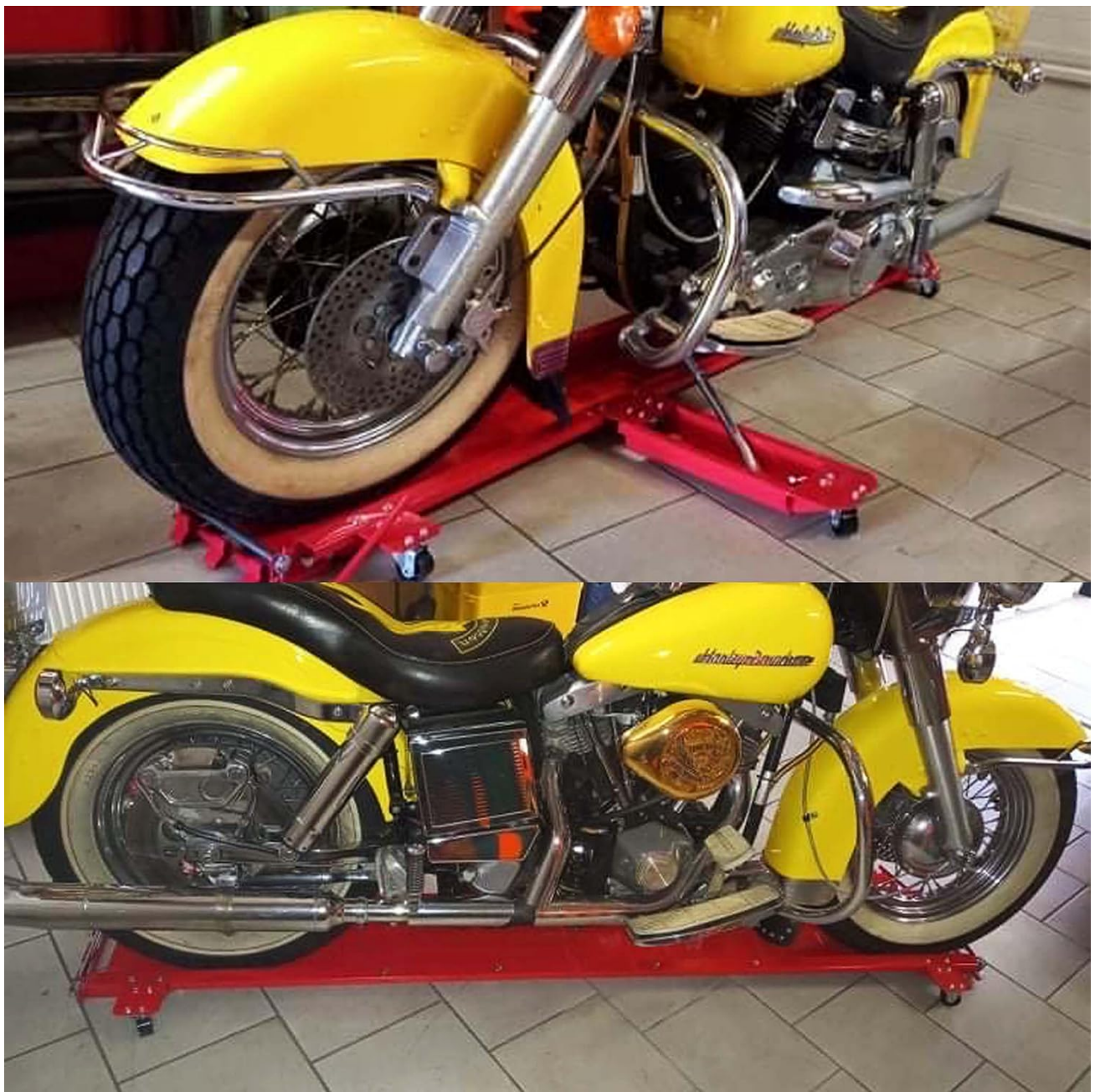
Figure 4: A yellow motorcycle positioned on the dolly, demonstrating how the side stand rests on the support arm.
