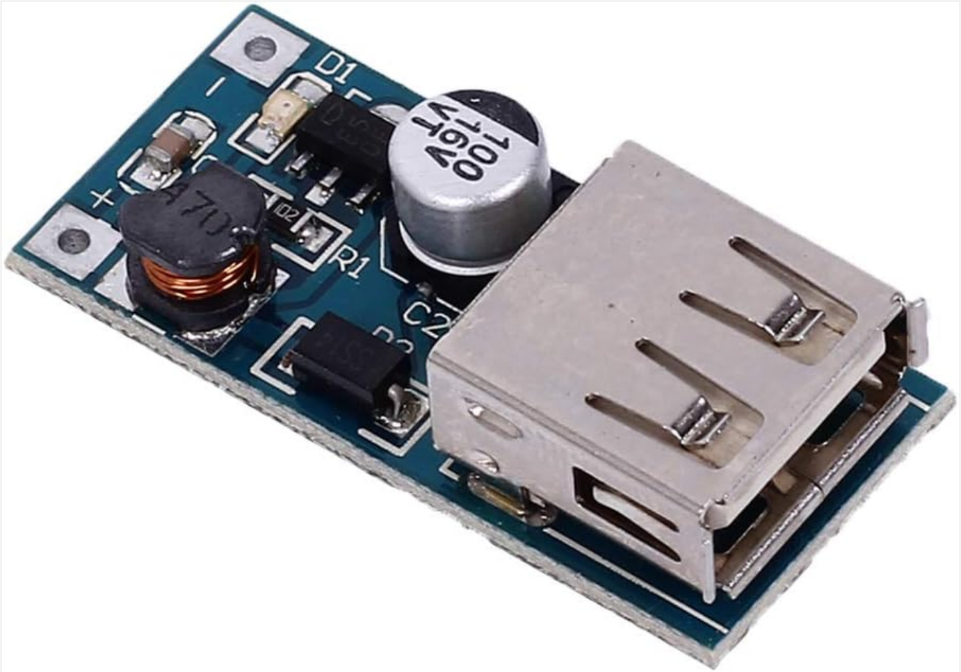
Figure 1: Top view of the ICStation USB DC-DC Step Up Power Supply Module, showing the USB output port and main components.
