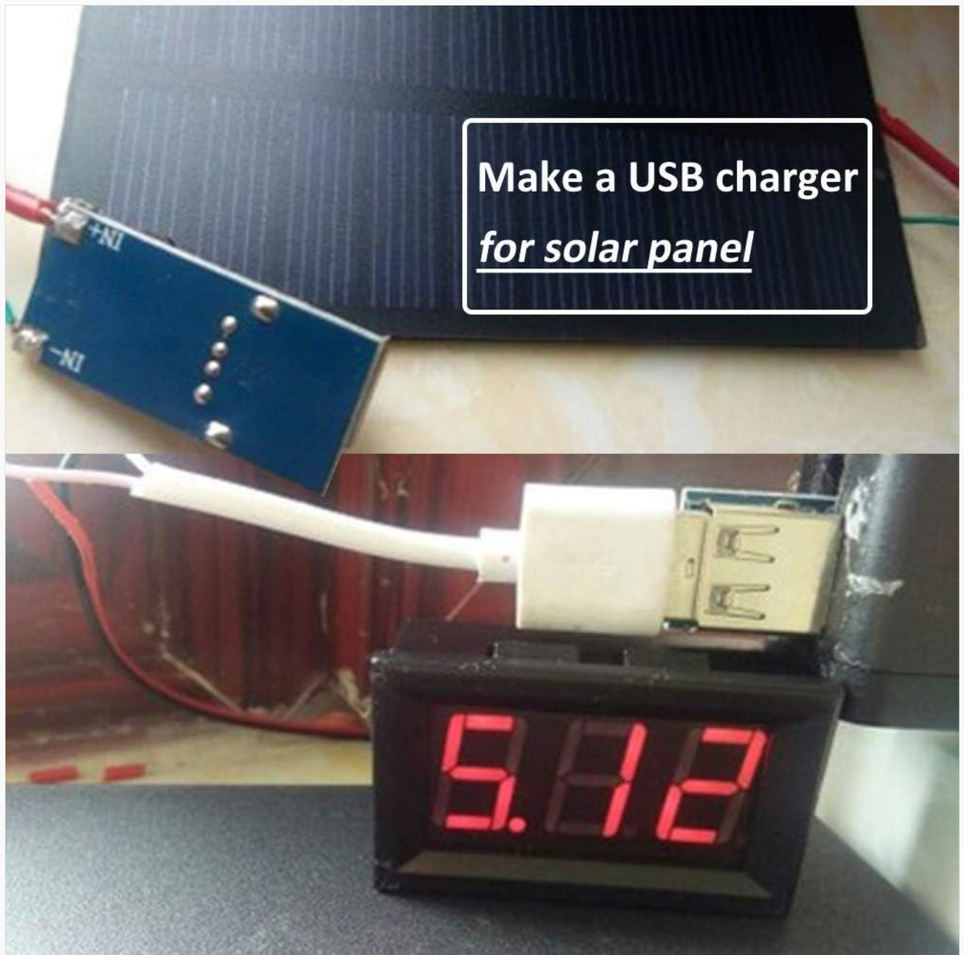
Figure 5: The module connected to a solar panel to provide 5V USB output for charging.
