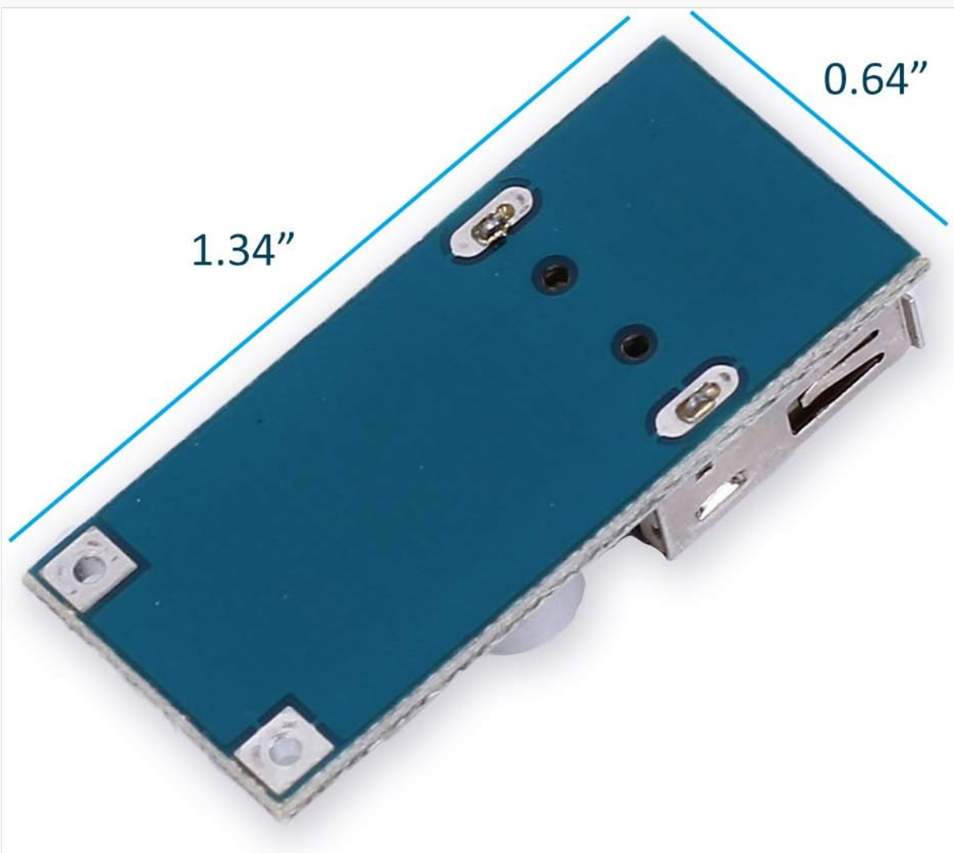
Figure 3: Physical dimensions of the module, approximately 1.34 inches by 0.64 inches.
