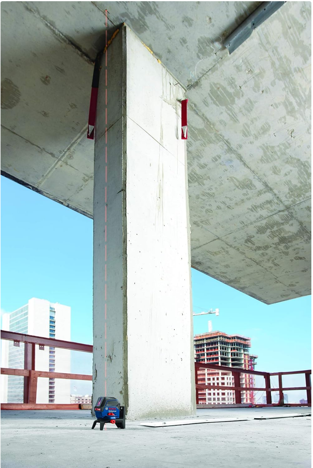
Figure 4: The four primary selection modes: Horizontal Laser Line, Vertical Laser Line, Horizontal & Vertical Laser Lines & Plumb Points, and Laser Plumb Points.
