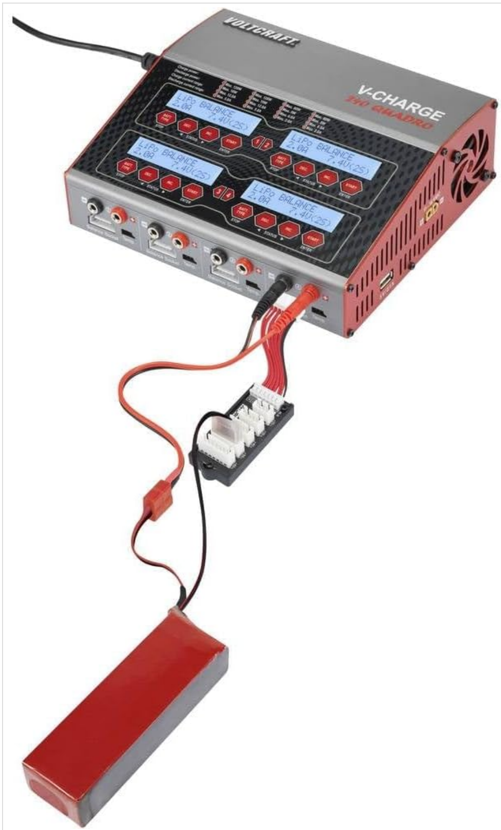
Figure 2: Front panel of the V-Charge 240 Quadro, highlighting the four charging channels with main output and balance ports.
