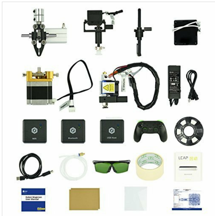
Figure 2.1: Overview of the various components and accessories included in the Dobot Magician kit.
