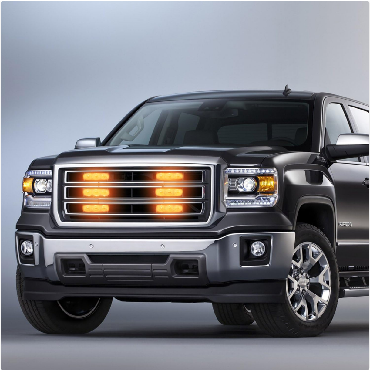
Figure 5.2: Example Installation. This image shows the FXC 3-LED Strobe Lights installed on the grille of a pickup truck, demonstrating a typical application.
