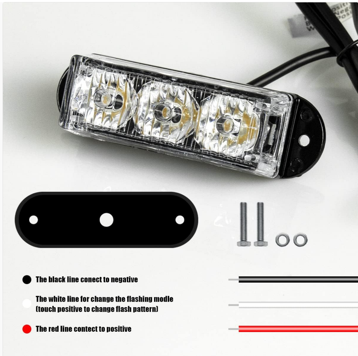
Figure 5.1: Wiring Diagram. This image illustrates the wiring connections for the FXC 3-LED Strobe Lights. The black wire connects to the negative pole, the red wire connects to the positive pole, and the white wire is used to change the flashing mode by momentarily touching it to the positive pole.
