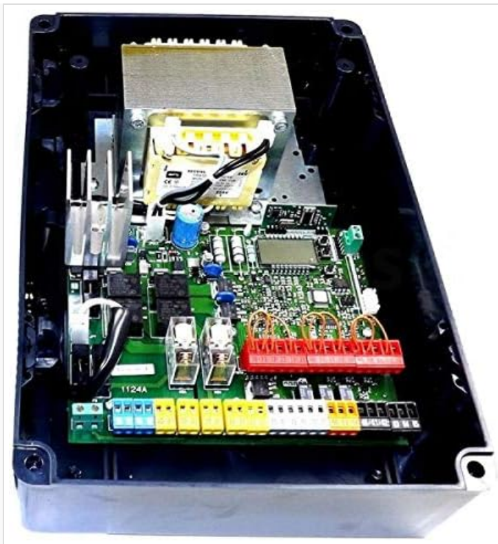
Figure 3: Detailed view of the THALIA P circuit board, highlighting the various terminal blocks for wiring connections.
