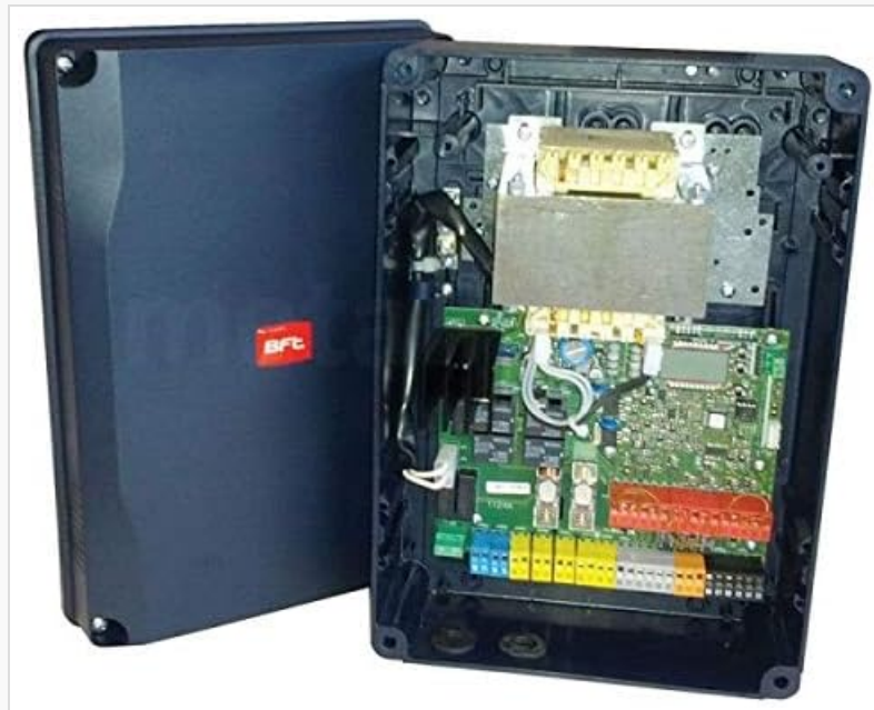
Figure 2: Internal view of the BFT THALIA P Control Panel with the cover removed, showing the circuit board and transformer.
