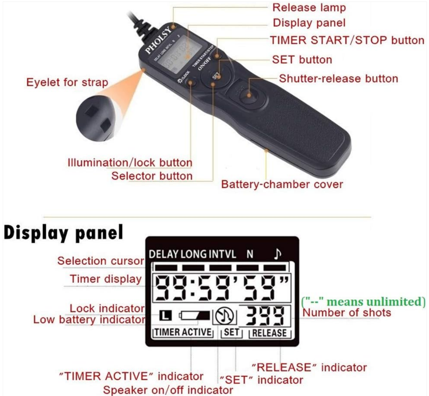
Figure 3: Labeled components of the PHOLSY S6 Timer Remote Control.
