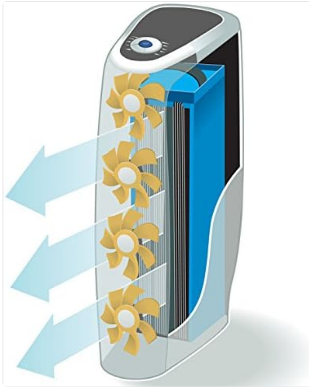
Image: An internal diagram illustrating the airflow path through the air purifier, highlighting the multiple fans and the filter system.
