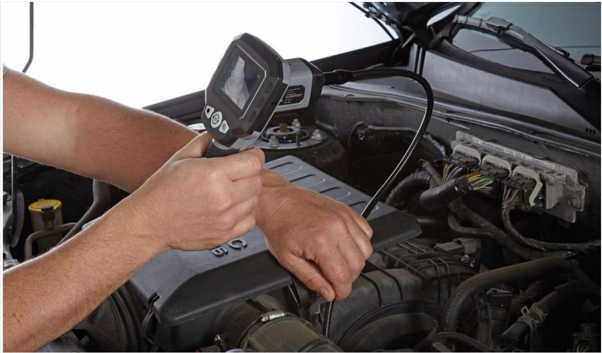
Image: The flexible cable allows for detailed inspection of engine components and other automotive areas.
