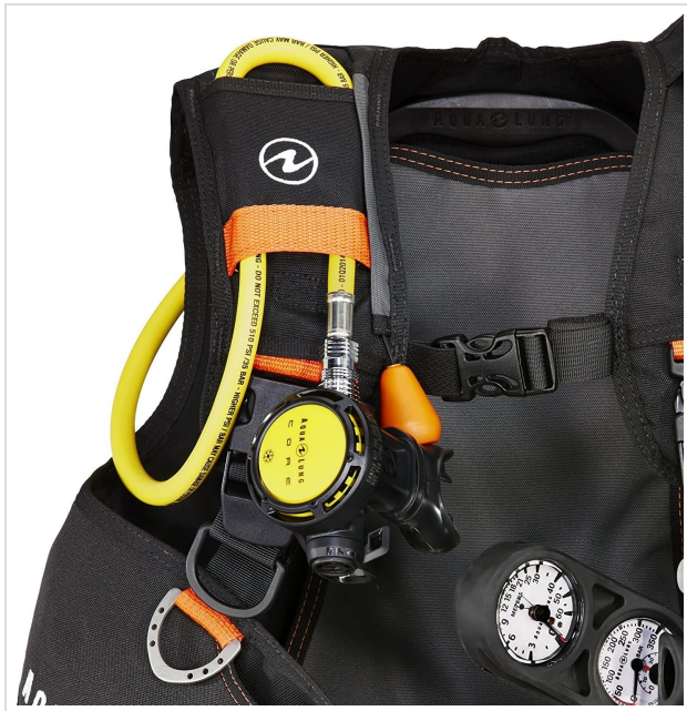
Figure 3.4: Detail of the right shoulder strap, featuring the octo-sleeve for an alternative octopus regulator placement. The inflator hose connection point and a D-ring are also visible.
