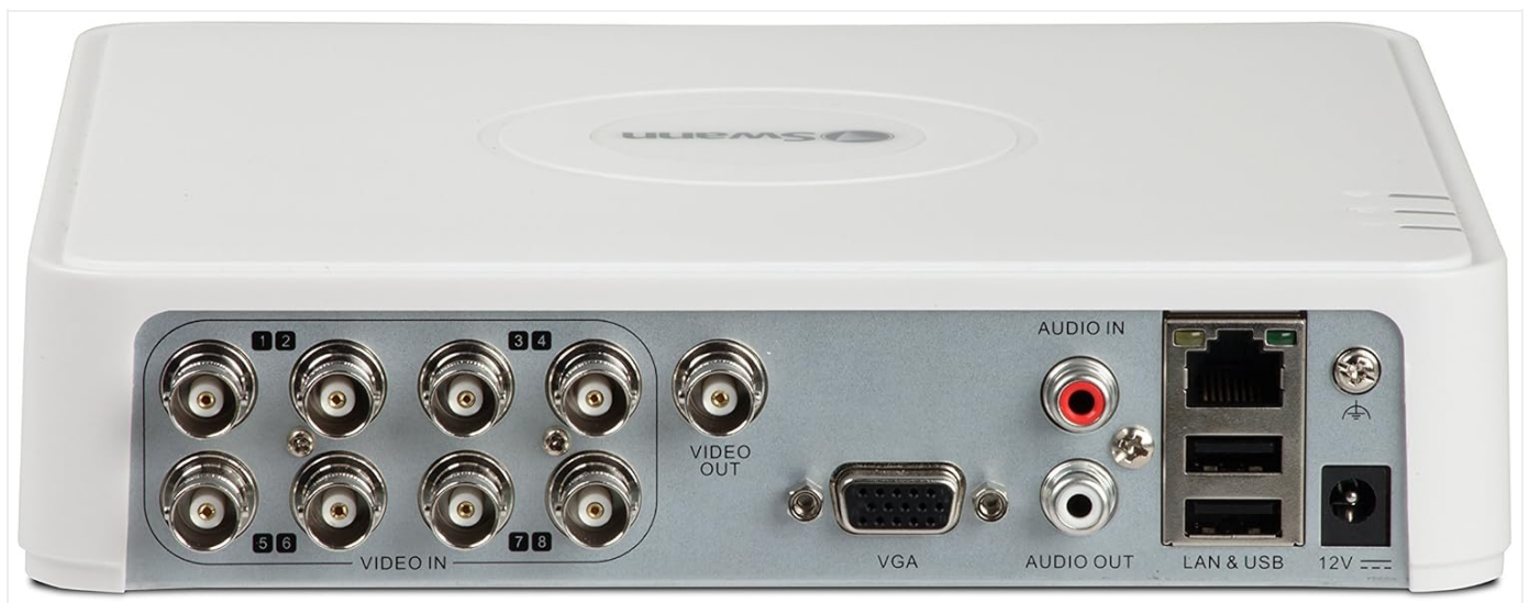
Figure 2: Rear Panel Connections of the SRDVR-81525H-US DVR. This view highlights the various input and output ports, including 8 BNC video input connectors (labeled 1-8), a BNC video out, VGA out, Audio In (RCA), Audio Out (RCA), LAN port, two USB ports, and the 12V DC power input.
