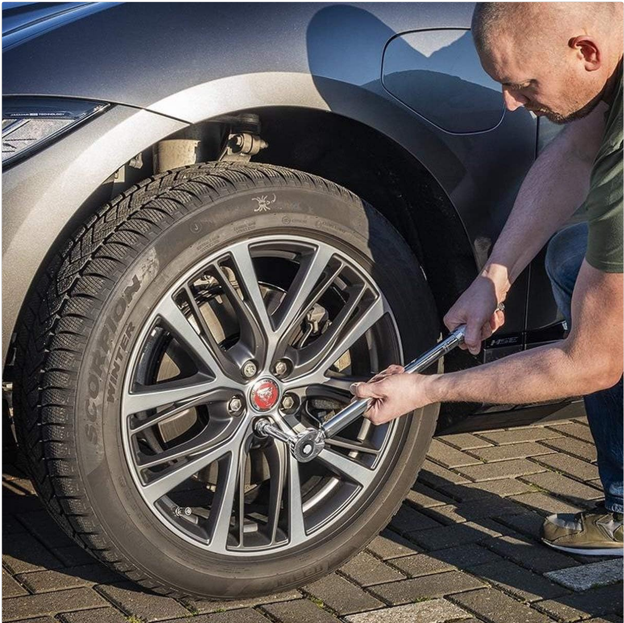
Image 5.1: A person demonstrating the use of the torque wrench to tighten lug nuts on a vehicle wheel, applying steady force.
