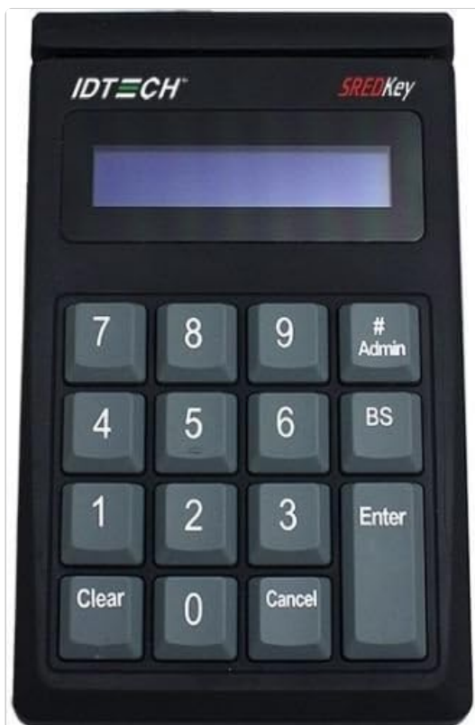
Figure 2.1: Front view of the ID TECH Keypad, showing the display, numeric keys (0-9), and function keys like 'Clear', 'Cancel', 'Enter', 'BS', and '# Admin'.
