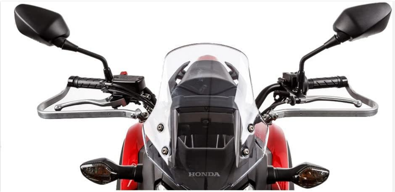
Figure 3: Front view of the handguard mounting kit installed on a motorcycle. This image demonstrates the overall appearance and positioning of the aluminum frames when mounted.
