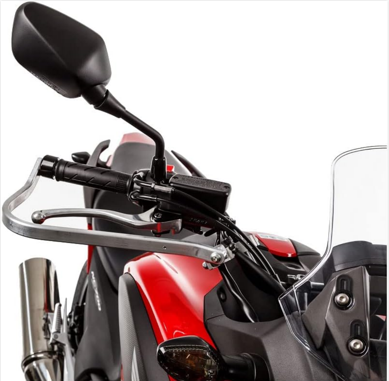
Figure 3: Front view of the handguard mounting kit installed on a motorcycle. This image demonstrates the overall appearance and positioning of the aluminum frames when mounted.
