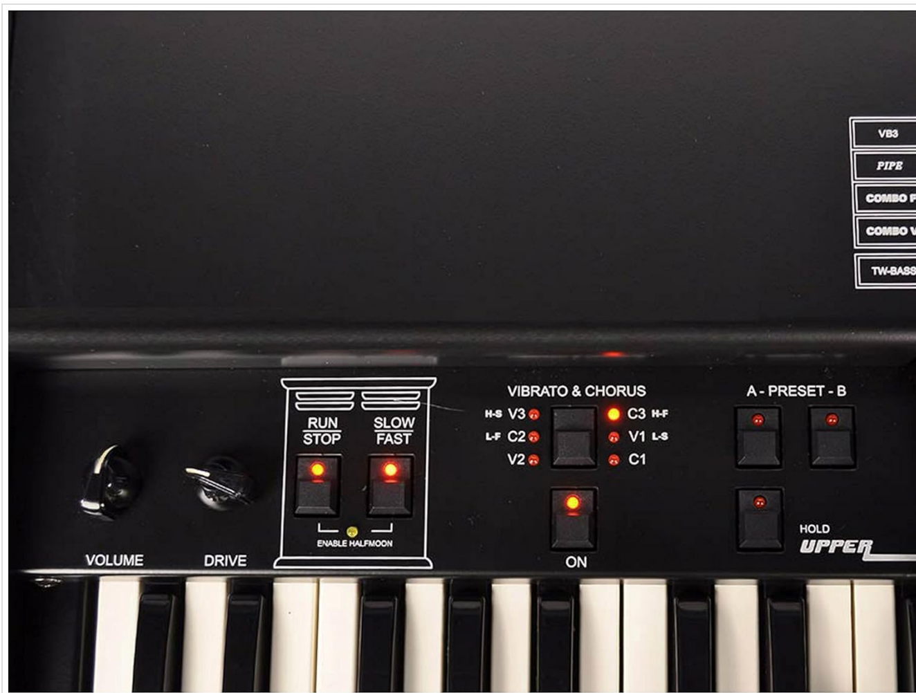
Figure 4.4: Detailed view of the Vibrato & Chorus section on the Crumar Mojo 61, showing the selector switches for various vibrato and chorus types (H-B V3, L-F C2, V2, C1) and the ON switch.
