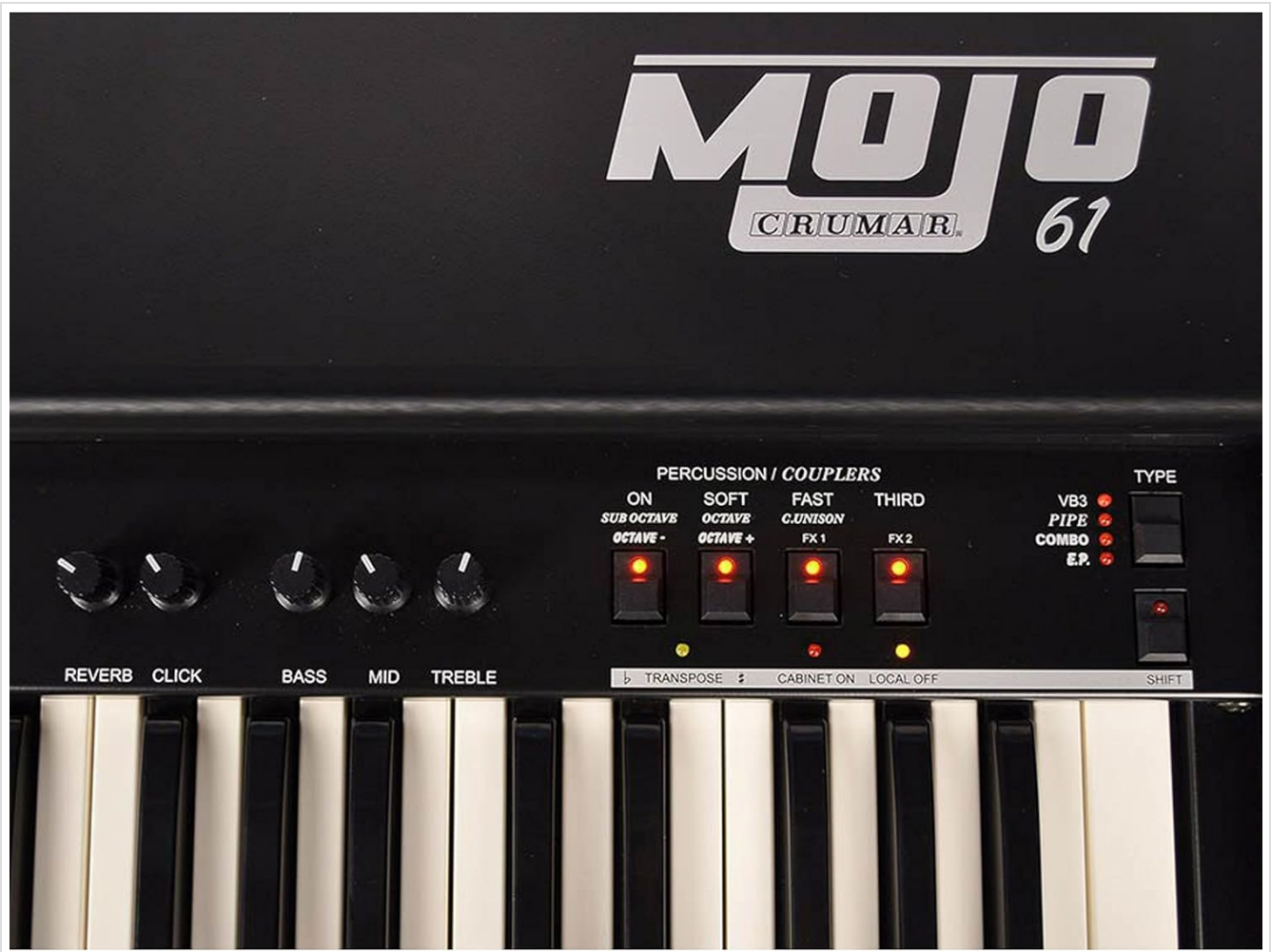
Figure 4.7: Detailed view of the Percussion/Couplers section and the Type selector (VB3, Pipe, Combo, E.P.) on the Crumar Mojo 61, including Transpose, Cabinet On, and Local Off switches.
