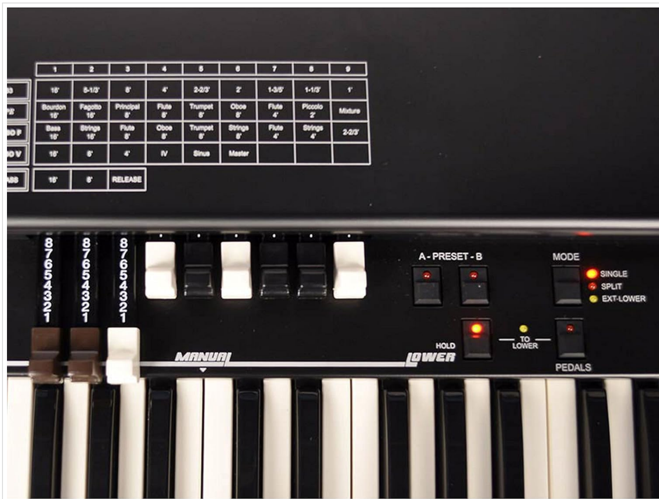
Figure 4.5: Close-up of the manual drawbars and the A-Preset-B, Mode, Hold Upper/Lower, and Pedals controls on the Crumar Mojo 61.
